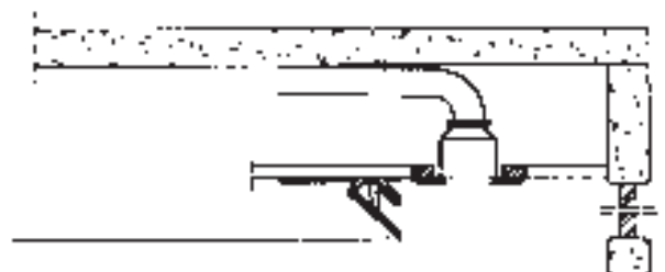
Air supply or extract system on glazed surfaces.
